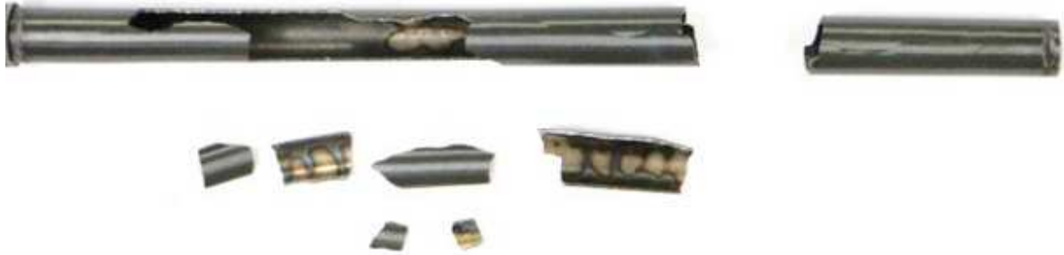
(a) Uncoated Zircaloy-4 clad segment, weight gain = 40,4 mg/cm 2
