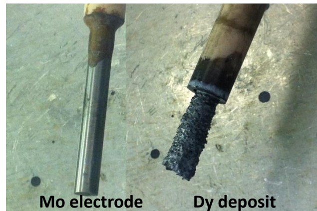
Metal deposition tests on the gram scale
