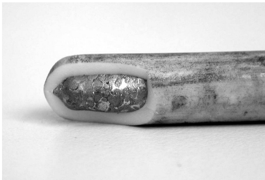
Figure 4: Details of the Bi/Bi 2 O 3 reference electrode featured on a broken sensor.
