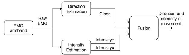
Fig. 3: General Approach (Intensity<sub>B</sub> and Intensity<sub>T</sub> correspond respectively to the intensity of the Biceps activation and Triceps activation)
