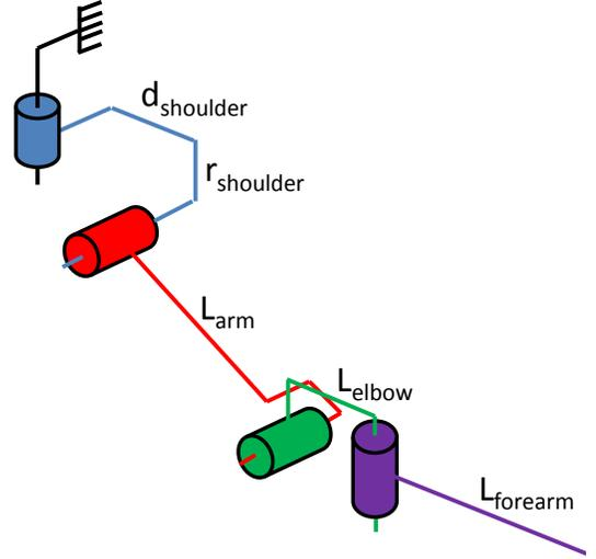
Fig. 2: Representation of the DHM parameters [14]
