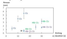
Fig. 6. Rmean for various etching durations and chemistries. These preliminary studies show that Rmean and Rmax values
