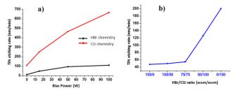
Fig. 3a and 3b. TiN etching rate in HBr and Cl<sub>2</sub> plasmas as a function of bias power (left), and of HBr/Cl<sub>2</sub> ratio (right).
