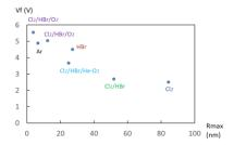
Fig. 8. Evolution of forming voltage Vf as function of R<sub>max</sub> for various chemistries. R<sub>max</sub>: maximum roughness.
