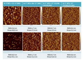
Fig. 4. AFM measurements performed at the center (top images) and at the edge (bottom images) for 4 various chemistries.
