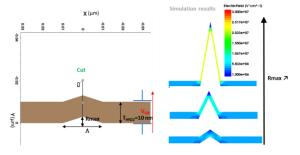
Fig. 10: Schematic of the defect simulating a microroughness on the TiN Bottom Electrode. A and  $R_{max}$  are respectively width and height of the micro-roughness.
