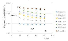
Fig. 12: Evolution of maximum electric field in  $HfO_2$  layer as function of  $\Lambda$  and of  $R_{max}$ . Applied voltage is 4 V.
