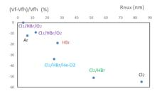
Fig. 9b. Evolution of the ratio (Vf-Vfh)/Vfh as function of the R<sub>max</sub>. Vf is the forming voltage at a given roughness, Vfh is the highest forming voltage obtained for the smallest value of R<sub>mean</sub> or R<sub>max</sub>.
