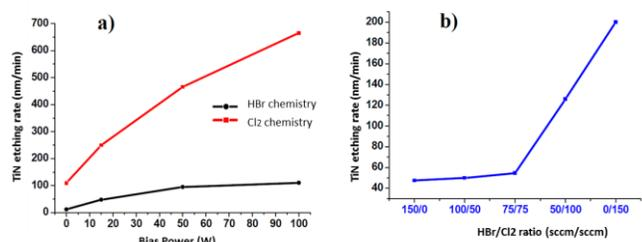
Fig. 3a and 3b. TiN etching rate in HBr and  $\text{Cl}_2$  plasmas as a function of bias power (left), and of  $\text{HBr}/\text{Cl}_2$  ratio (right).
