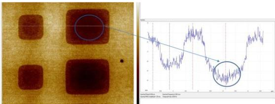
Fig. 11. AFM measurements for smooth samples (no-etching step).
