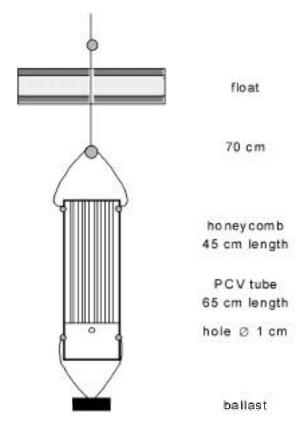
Figure 2. The suspended matter collector.
