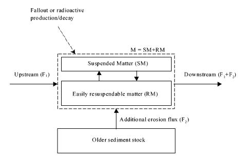
Figure 8. Simple steady-state fluxes and stocks model used to simulate suspended sediment transport in the lower river Seine.
