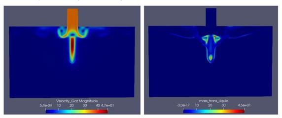
Figure 17: Velocity profile and liquid mass transfer in the LPWT at t = 0.57s
