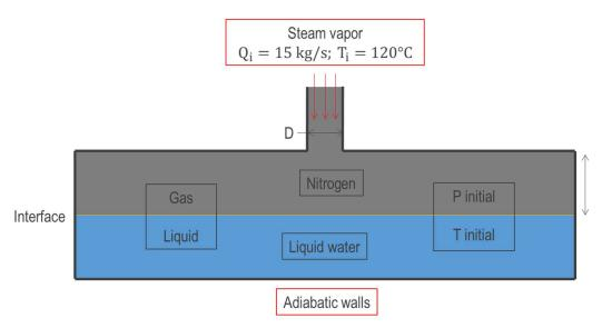
Figure 8: Initial and boundary conditions
