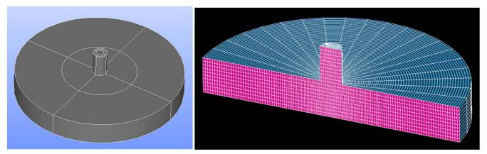
Figure 7: Geometry of the LPWT sectional view of the LPWT mesh
