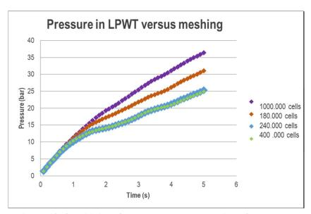
Figure 10: Sensitivity of the mesh on the evolution of the pressure
