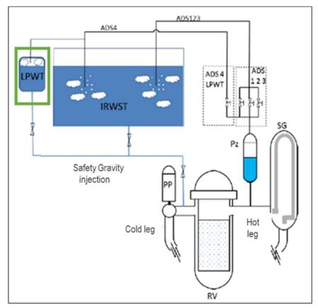
Figure 3: Passive safety system proposed by the CEA
