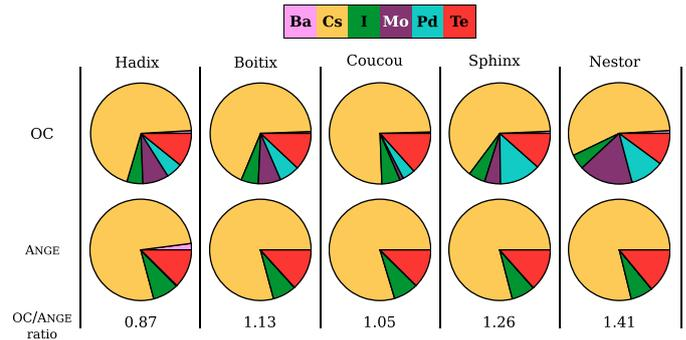
**Fig. 4.** Distribution of predicted released fission products in the different irradiation experiments described in Table 1. The bottom row is the ratio between the total released amount predicted by OC and ANGE. All data is taken from the maximum power node.
