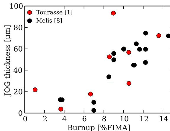
**Fig. 1.** Measured JOG thickness versus final burnup in some SFR fuel pins irradiated in the Phénix reactor. For reference [1], the burnup values refer to the local burnup at which the JOG was measured. For reference [8], the burnup refers to the maximum burnup reached in the fuel pin.
