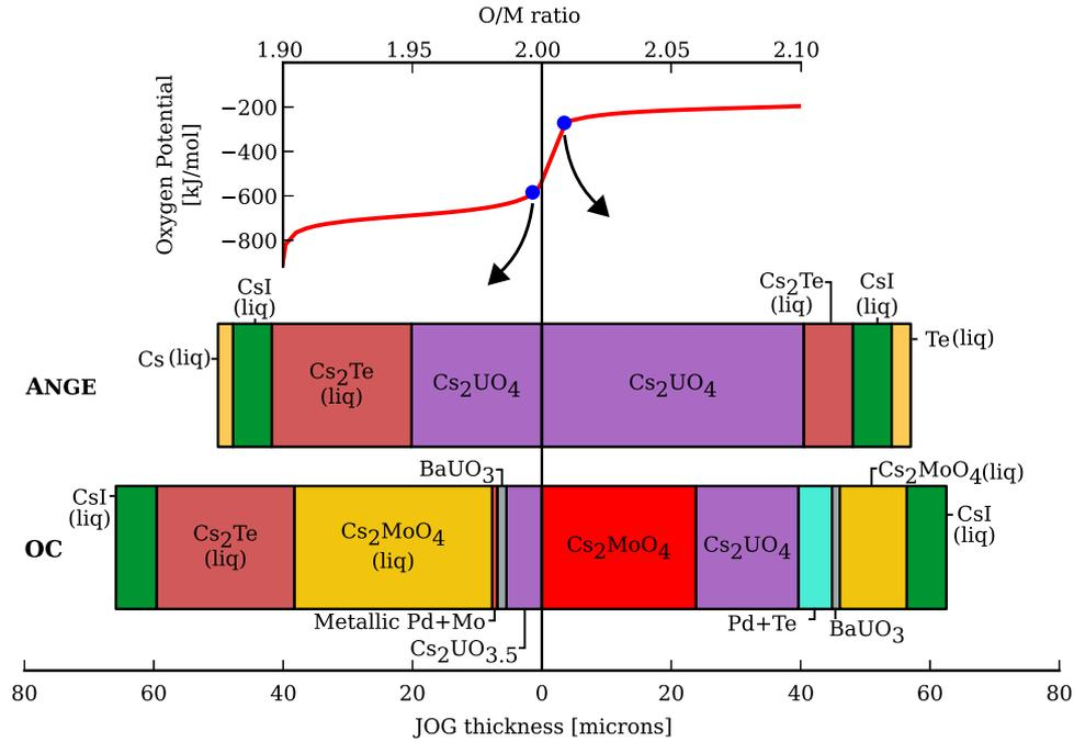
**Fig. 6.** JOG widths for the 13.4 %FIMA fuel pin calculated by OC and ANGE at 1000 K. The left case is just before the oxidation of Mo is complete, and the fluorite O/M ratio is just below 2. In the right case, oxygen amount has been slightly increased so that all Mo is oxidized, and the O/M ratio is just above 2.
