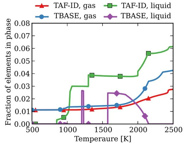
**Fig. 3.** Results from the test calculations of the 13.4 %FIMA fuel pin, mentioned in Section 3.2. For TAF-ID, OC has been used, and for TBASE, ANGE. It can be noticed that OC+TAF-ID predicts a higher fraction of liquid phases.
