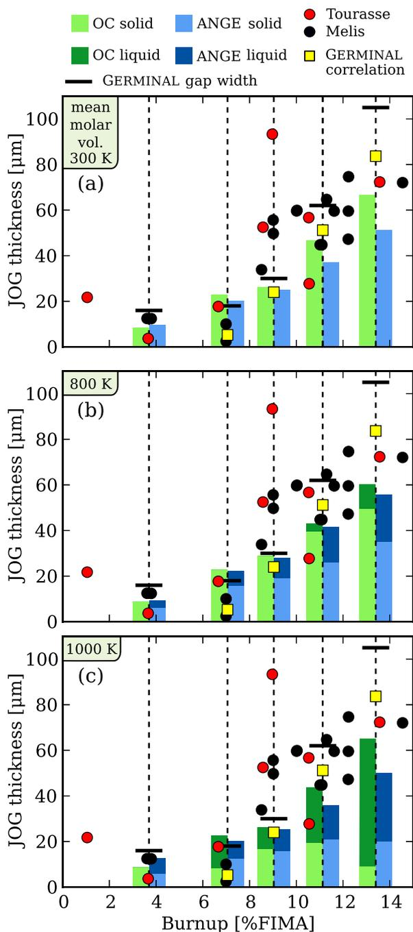
**Fig. 5.** JOG thickness predicted by ANGE and OC. In (a), a uniform molar volume corresponding to that of  $\text{Cs}_2\text{MoO}_4$  at room temperature has been assumed for all fission products. In (b) and (c) the gap composition has been evaluated thermodynamically at 800 K (b), and 1000 K (c). In Tourasse (red dots) [1], the burnup values refer to the local burnup at which the JOG was measured. In Melis (black dots) [8], the burnup refers to the maximum burnup reached in the fuel pin.
