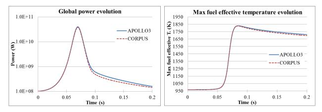
Figure 9. Total power (left) and max fuel effective temperature (right) evolutions during 2<sup>nd</sup> ejection.
