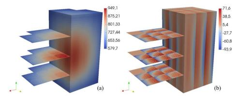
Figure 1. (a) Fuel effective temperature (K). (b) Fuel effective temperature difference (K) between one mean fuel rod per assembly and the calculation of every fuel rods.
