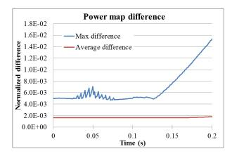
Figure 6. Power map max and average differences during 1<sup>st</sup> ejection
