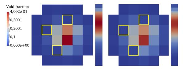
Figure 13. Final void fraction maps of the 2<sup>nd</sup> ejection (left: APOLLO3<sup>®</sup>, right: CORPUS)
