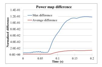
Figure 11. Power map max and average differences during 2<sup>nd</sup> ejection.
