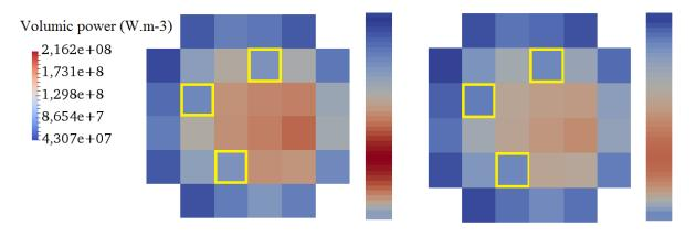
Figure 12. Final power maps of the 2<sup>nd</sup> ejection (left: APOLLO3<sup>®</sup>, right: CORPUS)
