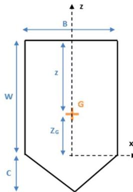
Figure 8: Notations for microscopic sample (pentagonal section)
