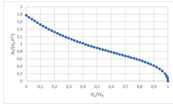
Figure 5: Critical stress evaluation from fracture stress
