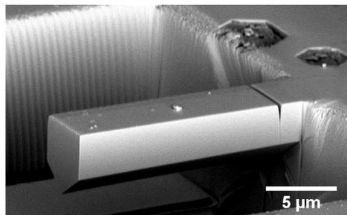
Figure 7: SEM image - Microscopic notched cantilever of fresh  $\text{UO}_2$
