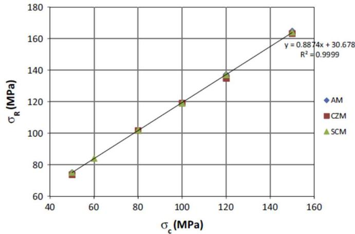
Figure 6: Comparison of the three approaches: Cohesive Zone Model, Smeared Crack Model and Analytical Model (respectively CZM, SCM and AM).
