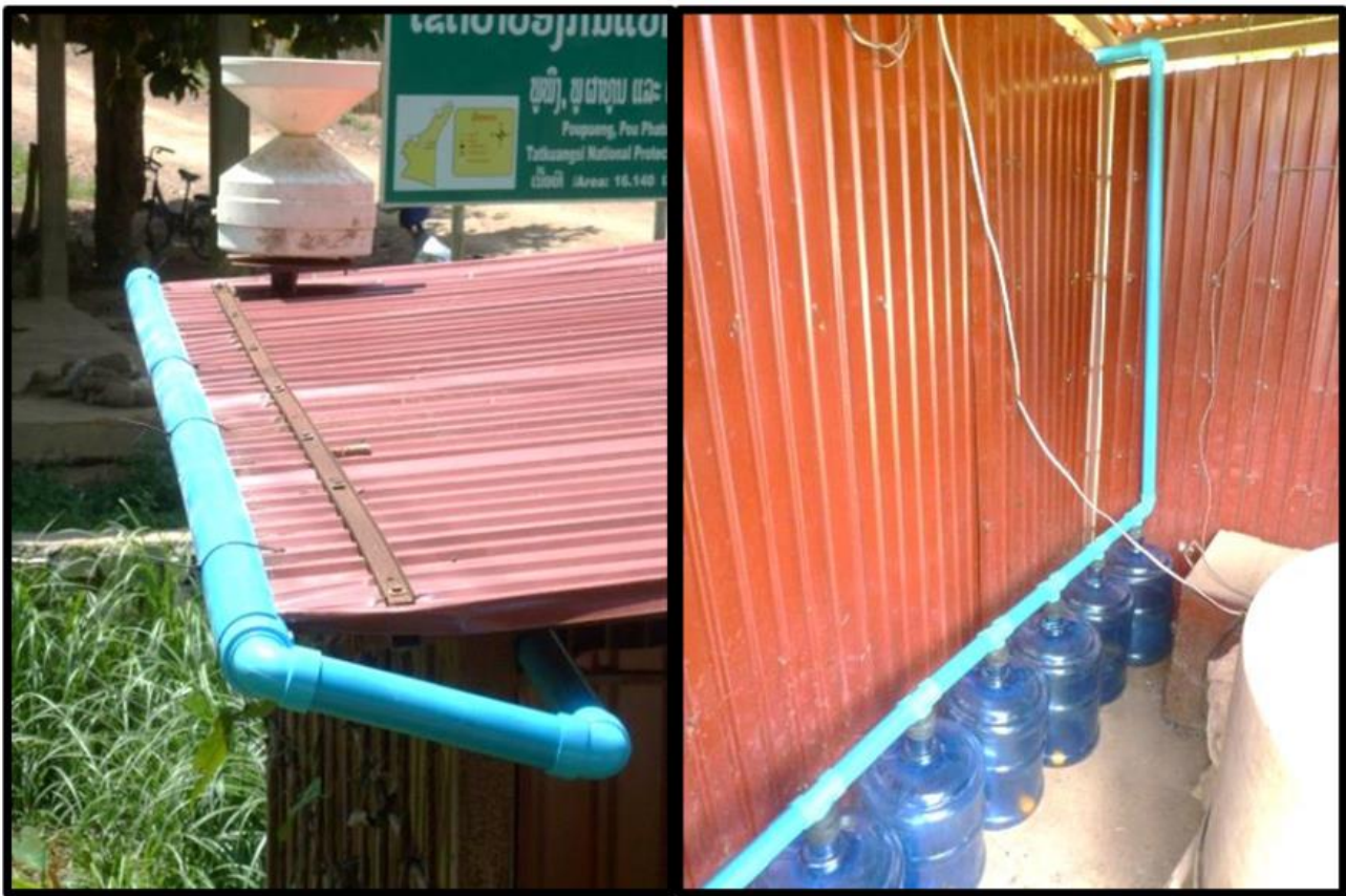
Fig. 2: Rainwater fractionated collection device at S10. left: pluviometer and collecting gutter; right: auto-capping 18L bottles connected to rainwater collection pipe.
