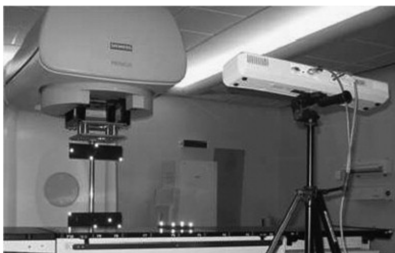
Fig. 2. The Polaris vision system used for patient positioning. This device is a binocular infra-red vision system able to detect 3D motions of markers reflecting infra-red light. These markers may be placed on the moving part of a phantom or on the skin of a patient.
