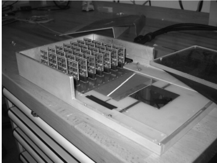
Fig. 10. Open view of the current DFC 2D silicon imager. This device includes a single 6 \times 6 \text{ cm}^2 detection module, while the final demonstrator will include nine of them.
