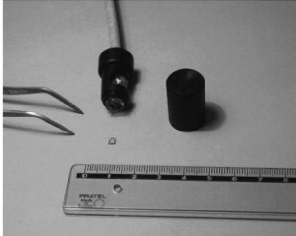
Fig. 8. TL (on the right) and diamond ionisation chamber (on the left).
