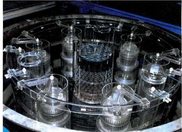
Fig. 5: Picture of the COLCHIX Plexiglas mockup for EFR
