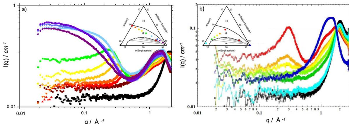
Figure 6: SAXS measurements along dilution lines, as shown on the phase diagrams with (a) increasing amount of oil (EA) (b) increasing amount of water.
