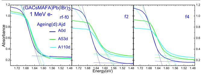
**Fig. 2** Bandgap determination from the energy dependence of absorbance (air, ~300 K) after aging in (GACsMAFA)Pb(IBr)<sub>3</sub> HOIPs for the reference Aid rf-f0 layer and the 1 MeV e-irradiated Aid fn layers
