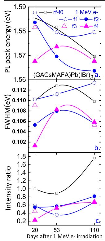
Fig. 3 Aging dependence of photoluminescence after 3-min illumination\_energy peak (a), FWHM (b), intensity ratio (c) in (GACsMAFA)Pb(IBr)<sub>3</sub> HOIPs for the reference Ajd\_rf-f0 layer and the 1 MeV e-irradiated Ajd\_fn layers at the fn fluence. The conditions for the Ajd aging are j(d) = 20/53/110 under N<sub>2</sub> atmosphere in dark at ~300 K. Laser Illumination is performed in (air, ~300 K) at the 454 nm wavelength and 11 W/cm<sup>2</sup> power density
