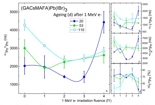
**Fig. 7** Fluence dependence of the average lifetime decay spectra recorded after aging and 30 min of laser illumination (Fig. 5) in (GACsMAFA)Pb(IBr)<sub>3</sub> HOIPs for the Ajd-rf-f0 reference layer and the Ajd\_fn 1 MeV e-irradiated layers at the fn fluence. The conditions for the
