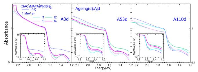
**Fig. 1** Energy dependence of Absorbance (air, ~300 K) after aging in (GACsMAFA)Pb(IBr)<sub>3</sub> HOIPs for the reference Ajd\_rf-f0 layer and the 1 MeV e-irradiated Ajd fn layers at the fn fluence. The conditions for the
