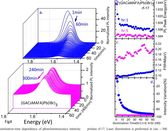
Fig. 4 Illumination-time dependence of photoluminescence intensity normalized to the background (a), energy peak (b), FWHM (c), intensity ratio (d) after aging in (GACsMAFA)Pb(IBr)<sub>3</sub> HOIPs for the
