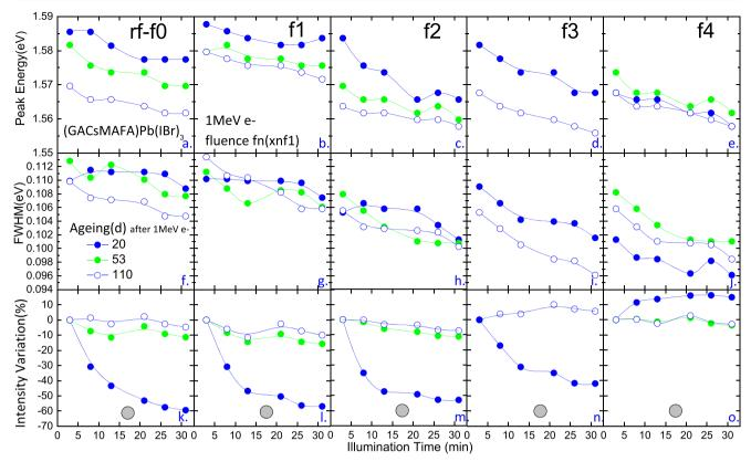
Fig. 5 Illumination-time dependence of photoluminescence\_energy peak (a–e), FWHM (f–l), intensity ratio (m–q) after aging in (GACsMAFA)Pb(IBr)<sub>3</sub> HOIPs for the Ajd\_rf-f0 reference layer and the Ajd\_fn 1 MeV e-irradiated layers at the fn fluence. The conditions for the Ajd aging are j(d) = 20/53/110 under  $N_2$  atmosphere in dark at  $\sim\!300~\text{K}$ .
