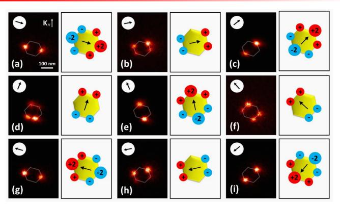
Figure 3 Polarization dependence of the dipolar plasmon mode of a 150 nm individual Au hexagon. Left column, PEEM imaging; right column, corresponding group theory predictions. Photon wavelength  $\lambda = 850$  nm, beam incidence angle  $\alpha = 72.5 \pm 2^{\circ}$ .
