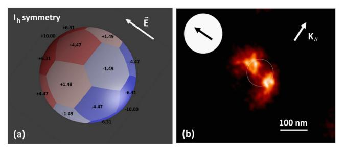
Figure 5 (a) Charge distribution of the dipolar plasmon mode in a sphere obtained using group theory (mesh grid in the form of a fullerene C<sub>60</sub> molecule, negative charge in blue, positive in red. (b) PEEM map of the dipolar plasmon field distribution of a Au nanosphere of 98 nm in diameter. Photon wavelength  $\lambda = 540$  nm, beam incidence angle  $\alpha = 72.5 \pm 2^{\circ}$ , *S* polarization.
