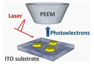
Figure 1 Schematic representation of the PEEM experimental setup
