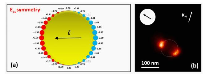
**Figure 4** (a) Charge distribution of the in-plane dipolar plasmon mode of a disk obtained using group theory (32 points mesh grid). (b) PEEM map of the dipolar plasmon field distribution of a thin Au nanodisk of 92 nm in diameter. Photon wavelength  $\lambda = 780$  nm, beam incidence angle  $\alpha = 72.5\pm2^{\circ}$ , 10° off *S* polarization.
