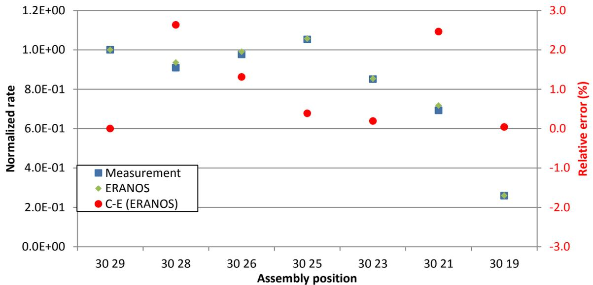
Figure 9. Measurement and ERANOS  $^{239}\text{Pu}$  fission rate at mid-height of the core.
