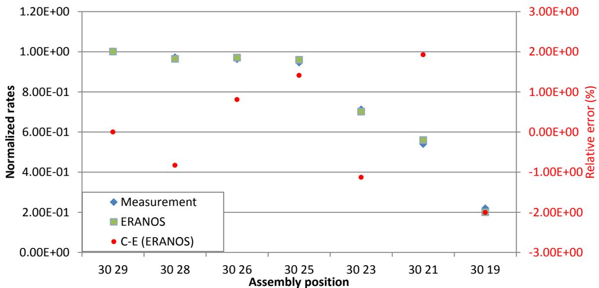
Figure 14. Measurement and ERANOS  $^{235}\text{U}$  fission rate at mid-height of the core.
