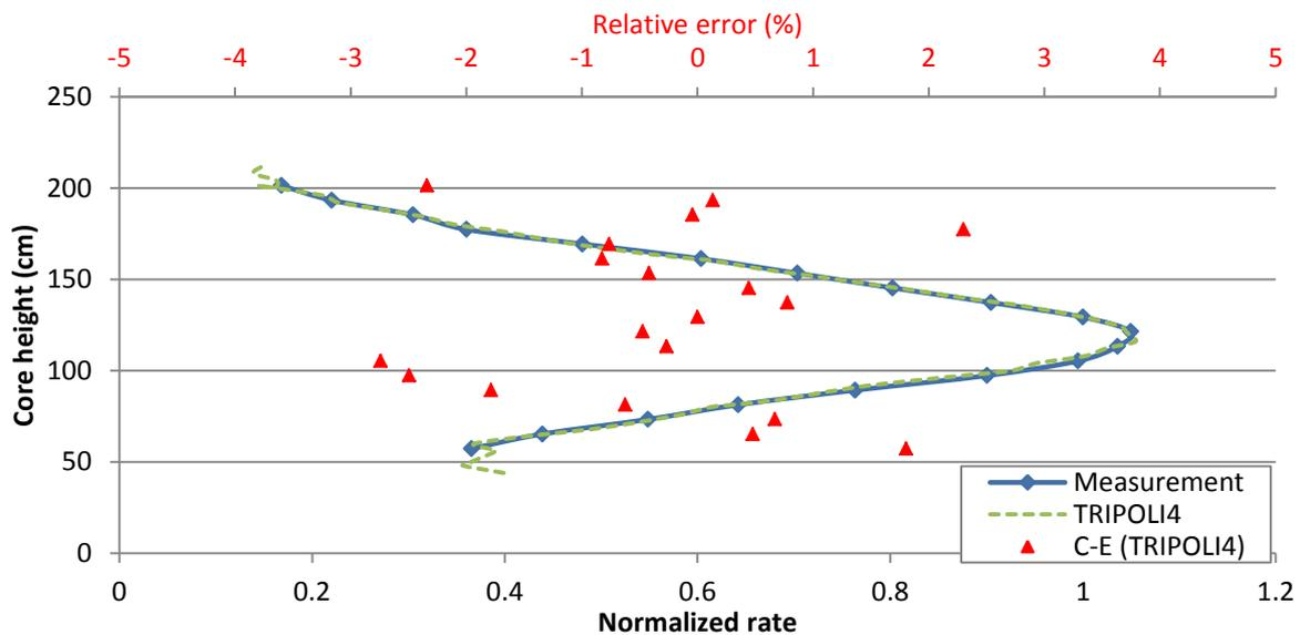
Figure 8. Measurement and TRIPOLI-4 axial <sup>239</sup>Pu fission rate for position 30 26.
