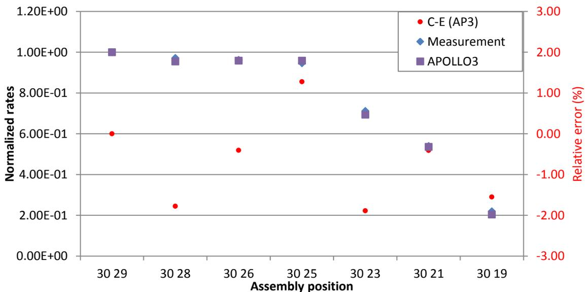
Figure 16. Measurement and APOLLO3 axial <sup>235</sup>U fission rate for position 30 26
