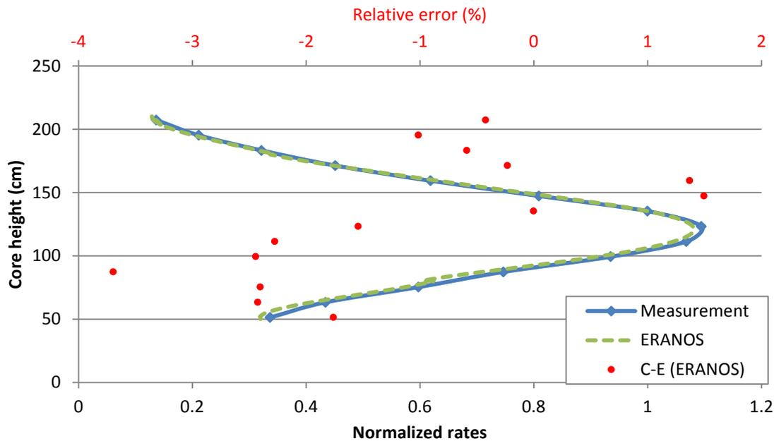
Figure 15. Measurement and ERANOS axial <sup>235</sup>U fission rate for position 30 26
