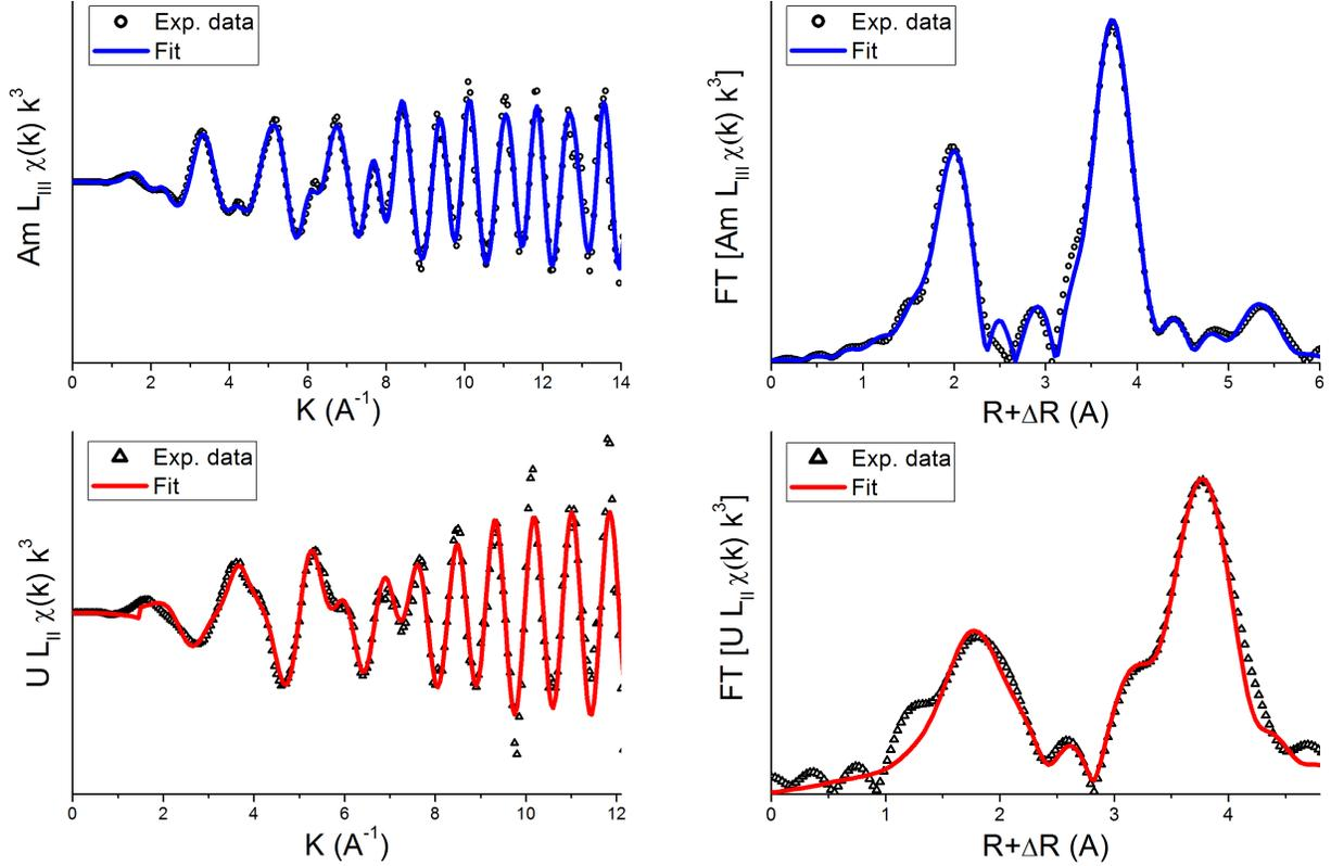
Figure 6: Am L<sub>3</sub> and U L<sub>2</sub> EXAFS spectra and Fourier transforms of the *Am50ox* sample. FT boundaries: 3.5-13.5 Å<sup>-1</sup>, dk = 2 Å<sup>-1</sup> for Am L<sub>3</sub>; 3.5-11.2 Å<sup>-1</sup>, dk= 2 Å<sup>-1</sup> for U L<sub>2</sub>.
