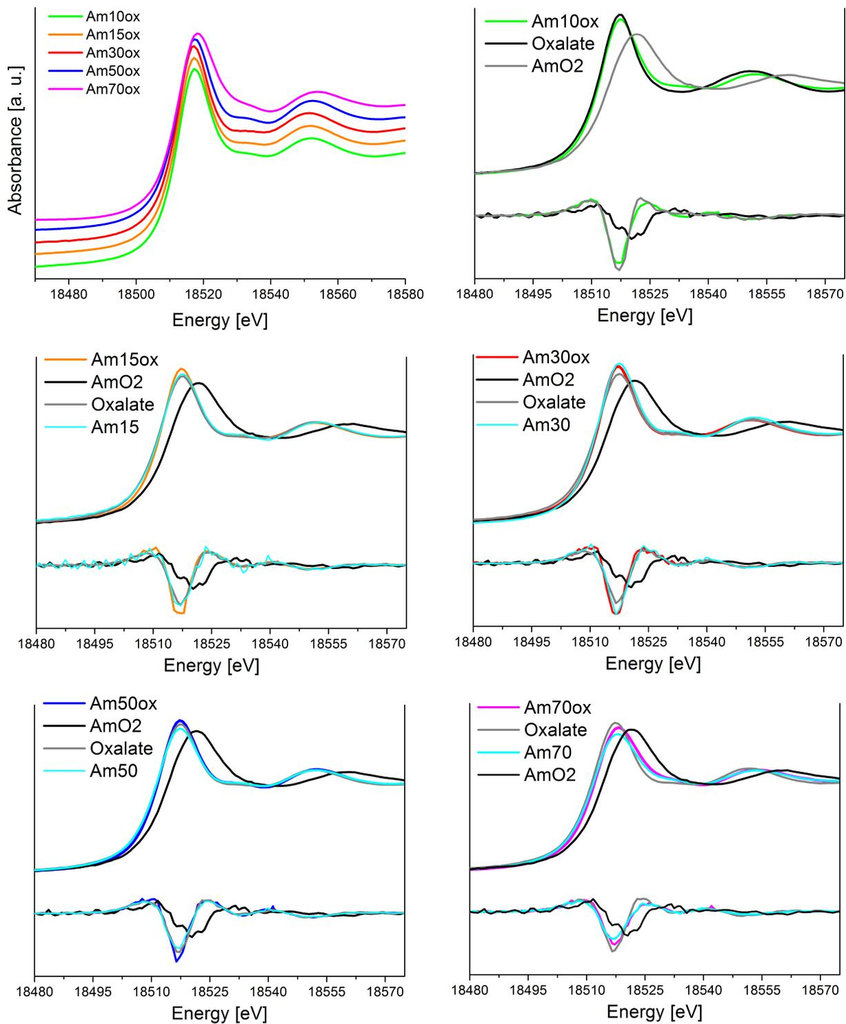
Figure 1: XANES spectra collected at the L<sub>3</sub> edge of Am and their second derivatives for the (U,Am)O<sub>2</sub> samples before and after oxidation in air.
