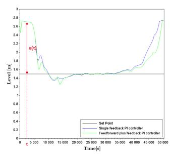
Fig. 7. Comparison of the two control strategies during an ideal sunny day with clear sky (no cloud passage)
