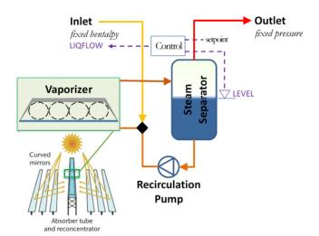
Fig. 2. Schematic view of the thermal-hydraulic sub-model.
