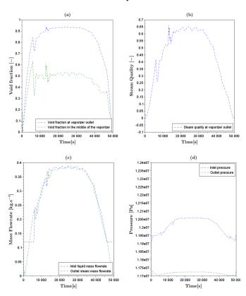
Fig. 5. Excerpts of the fluid thermal-hydraulic properties available from the co-simulation results (time evolutions over one day).
