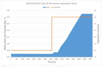
Fig. 6. Steam separator level identification test
