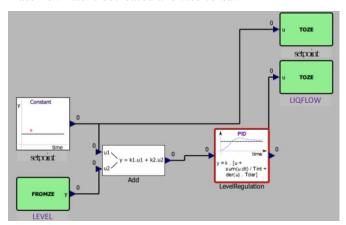
Fig. 4. View of the PI controller sub-model taken from the PEGASE framework.
