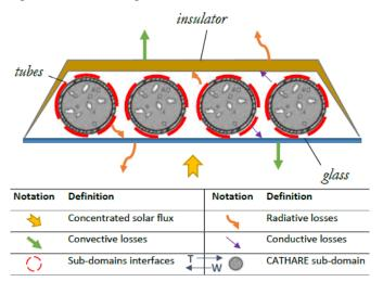
Fig. 3. Layout of a Fresnel Trapezoidal Receiver (FTR).
