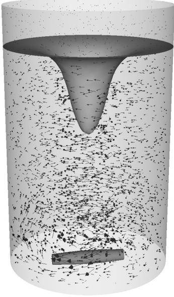
Figure 5: Nagata free-surface vortex and velocity vector field illustrating the initial state of the RVE.
