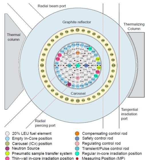
Fig. 1. Core configuration during the measurement campaign.
