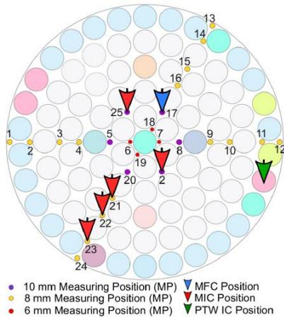
Fig. 2. Measurement positions inside the TRIGA core.
