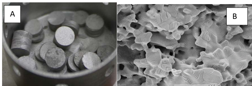
Figure 8: A) synthesized pellets (diameter about 8 mm) after carbo-reduction cycle and B) surface micrograph observed by SEM
