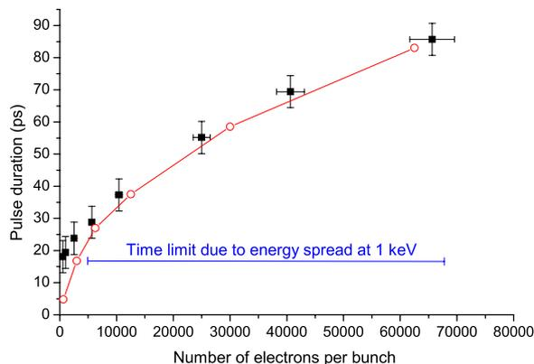
**Figure 2.** Computed (in red) and measured (in black) electron bunch temporal width as a function of the number of electrons per bunch, for 1 keV electrons and for a 600  $\mu\text{m}$  laser beam diameter on the photocathode.
