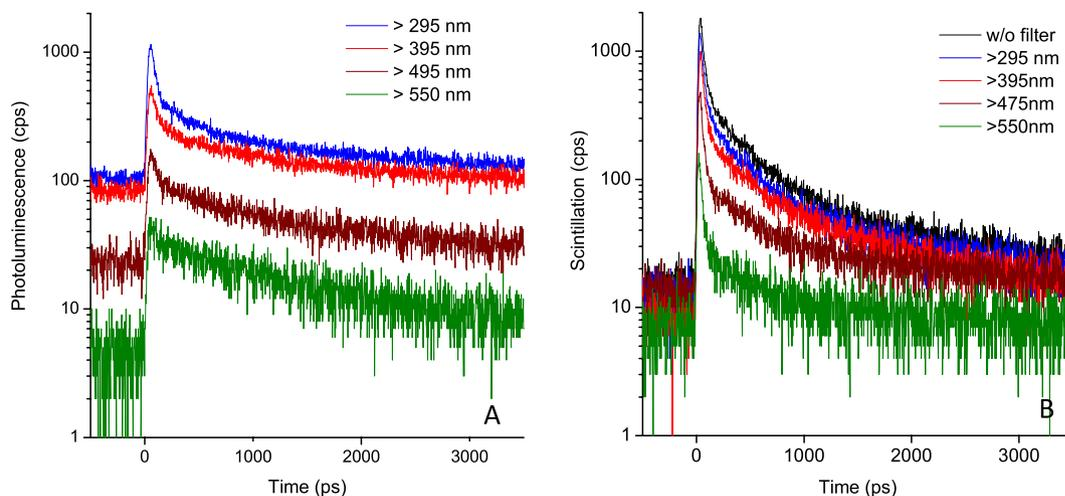
**Figure 4.** (A) Time-resolved photoluminescence of DNA film (TR-PL) and (B) time-resolved cathodoluminescence (TR-CL) of the same type of DNA film. The photoluminescence data could not be obtained without filter due to the strong 266 nm background.
