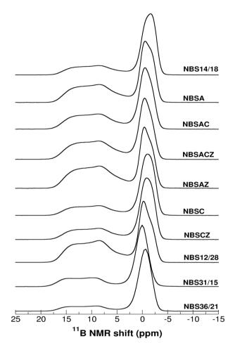
Fig. 2 11B MAS NMR spectra of all borosilicate glasses investigated in this study. Spectra are normalized to the B4 peak (centered around 0 ppm).
