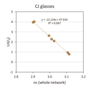
Fig. 3 Forward dissolution rate as a function of the number of constraints per atom  $(n_c)$  for the 7 borosilicate glasses selected to train the model (training set, CJ series, see Table 1). The data are fitted by Eq. 1. The standard deviation on the slope is 0.356.
