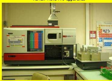
Seaspray nebulizer, cyclonic chamber, axial view, CCD detector
