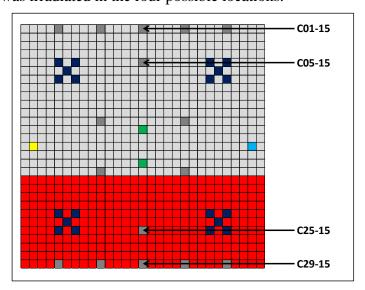
Figure 5: fission chamber loading
