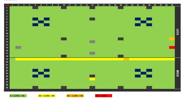
Figure 2: neutron source distribution validation
