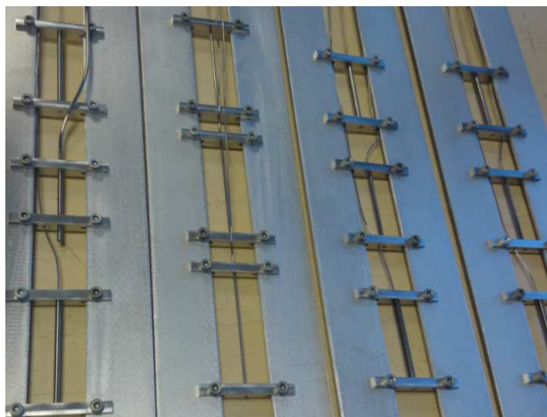
Figure 2. Photograph of the aluminium VASCO SPD holders with SPDs mounted in threes.
