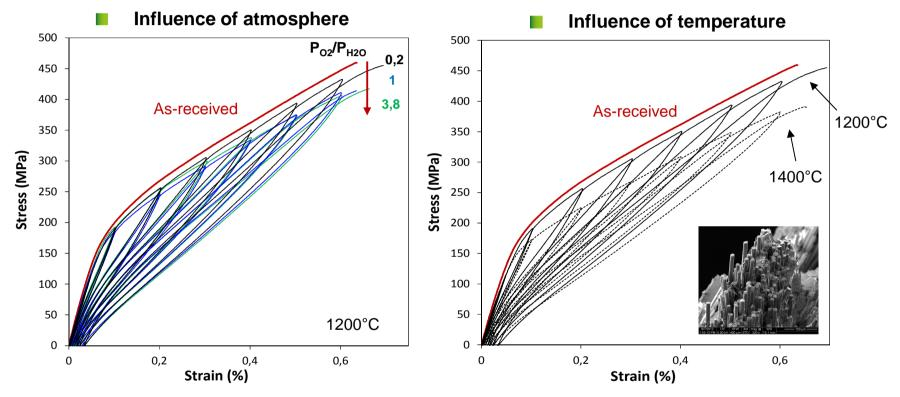
Retention of the characteristic « non-linear elastic damageable » behavior of CMCs (No reduction of strain to failure / Slight decrease of tensile strength and Young modulus)
