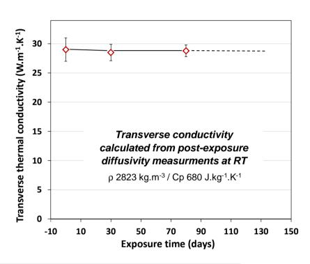
No effect of oxidation on the thermal behavior after 80 days
