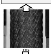
As-received and intentionally pre-damaged SiC/SiC at different level (0.05 to 0.5 %  $\sigma_{\text{R}})$
