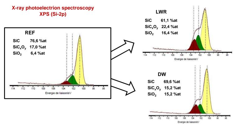
▶ After oxidation, presence of a larger (but low) quantity of SiO₂ oxide Surface is mainly composed of SiC after oxidation in both DW/LWR conditions
