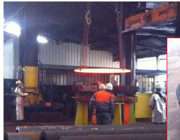
Heat Exchanger in-factory forging: Bottom part (November 2014)
