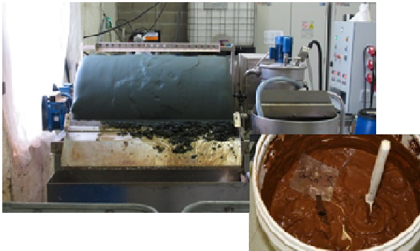
Fig. 2: Waste reconstitution: filtration, and photo of sludge before cementation
