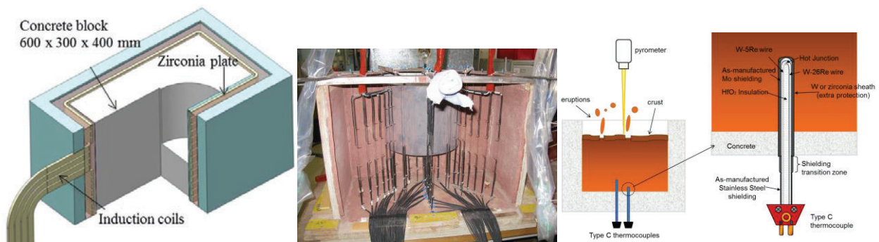
Figure 13. MCCI VULCANO concrete test section
