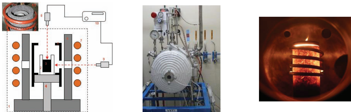
Figure 1. VITI experimental assembly for heating test in a crucible [3]: (1) VITI chamber, (2) crucible, (3) sample, (4) support for crucible, (5) graphite susceptor, (6) thermal shield, (7) induction coil, (8) pyrometer for sample temperature, (9) pyrometer for crucible temperature, (10) data acquisition, (11) picture of the assembly.
