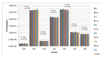
Fig. 7. Xe Isotopic ratio evolution as a function of time during 5 hours. (AV and SD stand for average et standard deviation respectively)
