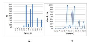
Fig. 3. Isotopic Xe spectrum: reference NIST spectrum (a) and spectrum recorded before calibration (b).
