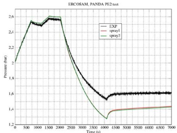
Fig.16. Post-test calculations of depressurization caused by spray in test PE2 with: (top) GOTHIC; (middle) FLUENT and various model choices; (bottom) with the LP code ASTEC (assuming two droplet trajectories).
