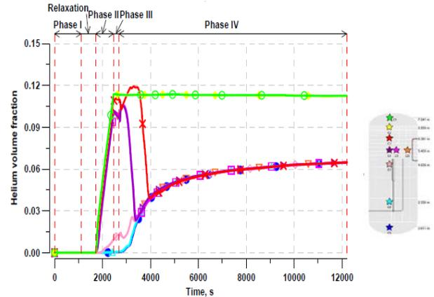
Fig.5. Planning calculations with KUPOL: helium concentrations at various elevations for test S1 in SPOT.
