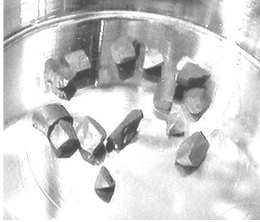
Fig. 12: Illustration of some UO_2 fragments pellet being extracted from pin CEA 7
