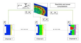
Figure 3 : Data exchange topology for the SIMMER-III/SNATCH coupled code
