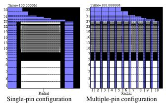
Figure 8: Radial meshing refinement (fuel bundle)
