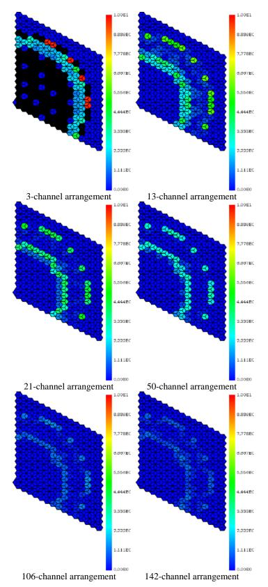
Figure 7: Absolute deviations of the averaged fuel-melt fraction with respect to the reference calculation
