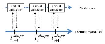
Figure 4: Strategy for obtaining the nominal state of a reactor
