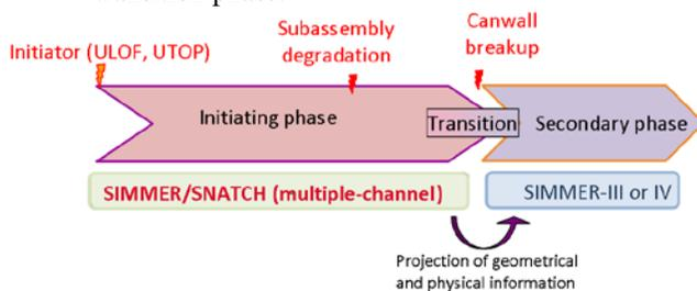
**Figure 2 : Alternate computational route for severe accident**
