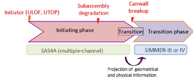
**Figure 1: Standard computational route for severe accident**
