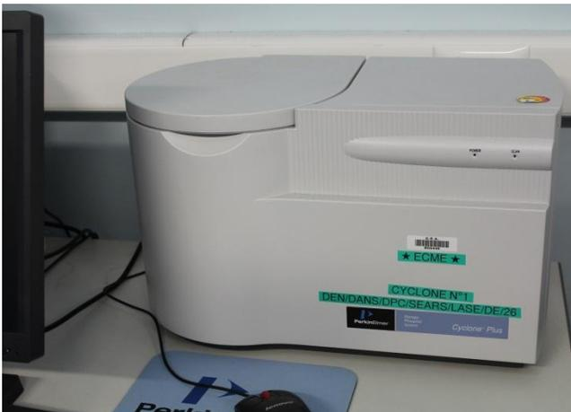
Fig. 3. Picture of the screen scanning device "Cyclone Plus" by Perkin Elmer; scanning time at worst resolution ( $169\ \mu\text{m}$ ) is 4 minutes
