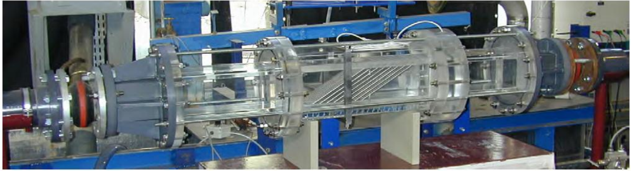
Fig. 1: EOLE test section with a tube bundle inclined at 30^\circ .
