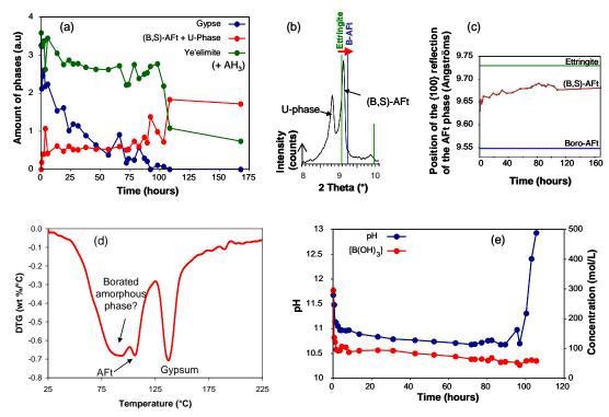
Figure 7 Hydration of a CSA cement by a sodium borate solution ([B] $_{tot}$  = 1 mol/L, pH = 11, w/c = 0.6, T = 20°C). (a) Mineralogical evolution inferred from XRD analysis. (b) Shift of the {100} reflection of the precipitated AFt-type phase compared to ettringite and B-AFt. (c) Evolution of the position of the {100} reflection of the (B, S)-AFt phase during hydration. (d) TGA analysis of a 24h-old sample. (e) Evolution of pH and boron concentration of the pore solution during hydration.
