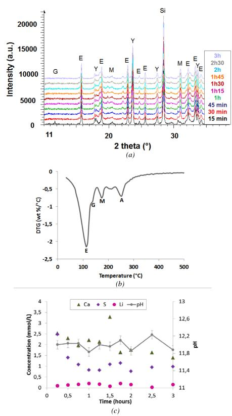
Figure 4 Hydration of CSA cement with 10% gypsum in the presence of a lithium hydroxide solution (Li/C = 0.03 mmol/g of cement, w/c = 0.6, T = 20°C) at early age : (a) X-ray diffraction patterns (E = ettringite, G = gypsum, M = monosulfate, Y = ye'elimite, Si = silicon); (b) TGA analysis of a 5 minute-old sample (E = ettringite, G = gypsum, M = monosulfate, A = aluminum hydroxide); (c) Evolution of pH and composition of the pore solution  $3.1.3 \ Discussion: possible mode of action of lithium$
