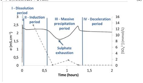
Figure 1 Evolution of the electrical conductivity during hydration of CSA cement by a 1 mmol/L lithium hydroxide solution ( $w/c=10,\,T=25^{\circ}C$ )
