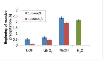
Figure 2 Time of occurrence of the massive precipitation period when CSA cement is hydrated by different mixing solution (salt added at a concentration of 1 or 10 mmol/L, w/c = 10, T = 25°C)
