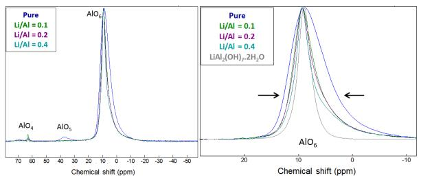
Figure 5 <sup>27</sup>Al-MAS NMR spectra of aluminum hydroxide (synthesized in the absence and in the presence of lithium) and of hydrated lithium aluminate LiAl<sub>2</sub>(OH)<sub>7</sub>.2H<sub>2</sub>O
