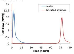
Figure 6 Heat flow produced during the hydration of CSA cement by water or by a sodium borate solution ( $[B]_{tot} = 1 \text{ mol/L}$ , pH = 11, w/c = 0.6, T = 25°C)
