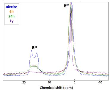
Figure 8  $^{11}$ B-MAS NMR spectra of ulexite and of cement paste samples hydrated by a sodium borate solution after 6 h, 24 h and 1 year. ([B]<sub>tot</sub> = 1 mol/L, pH = 11, w/c = 0.6, T = 20°C)
