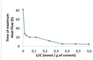
Figure 9 Heat flow recorded under isothermal conditions: influence of the initial LiOH concentration in the mixing solution on the hydration of a CSA cement hydrated by a sodium borate solution ([B]<sub>tot</sub> = 1 mol/L, pH = 11, w/c = 0.6, T = 25°C)
