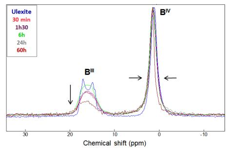
Figure 12 Comparison of the  $^{11}B$ -MAS NMR spectra of synthetic well-crystallized ulexite and of cement pastes hydrated by a sodium and lithium borated solution ([B]<sub>tot</sub> = 1 mol/L, Li/C = 0.03 mmol/g, pH = 11, w/c = 0.6,  $T = 20^{\circ}C$ )
