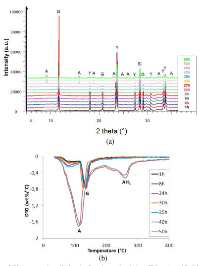
Figure 10 Hydration of CSA cement by a lithium/sodium borated solution ([B] $_{tot}$  = 1 mol/L, Li/C = 0.03 mmol/g, pH = 11, w/c = 0.6, T = 20°C) at an early age : (a) X-ray diffraction patterns (A = AFt phase, G = gypsum, Y = ye'elimite, Si = silicon); (b) TGA analyses (A = AFt phase, G = gypsum, AH $_3$  = aluminum hydroxide)
