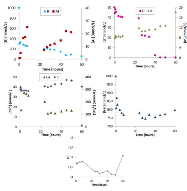
Figure 11 Hydration of CSA cement by a lithium/sodium borated solution ([B]<sub>tot</sub> = 1 mol/L, Li/C = 0.03, pH = 11, w/c = 0.6, T =  $20^{\circ}$ C) at an early age: evolution of pH and composition of the pore solution during hydration
