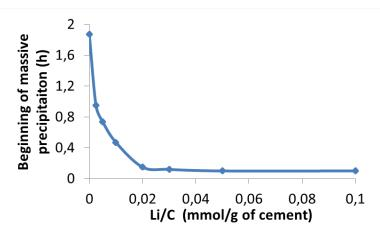
Figure 3 Time of occurrence of the massive precipitation period when CSA cement is hydrated by lithium hydroxide solutions of increasing concentration (w/c = 10, T = 25°C)
