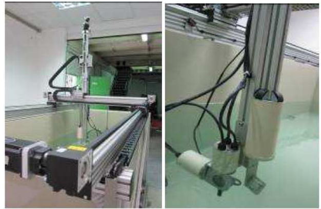
Fig. 25. VISIO water facility (2 m long, 1 m large, 1 m high) devoted to ultrasonic visualization study.
