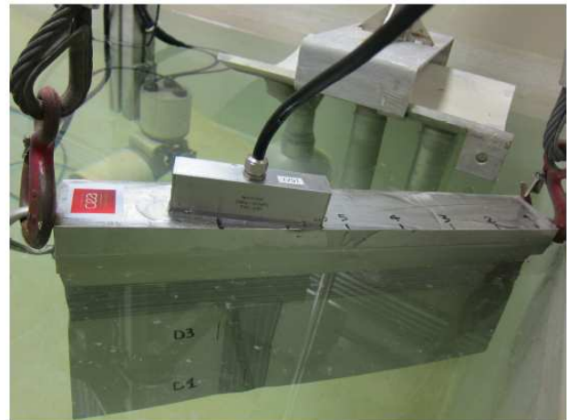
Fig. 19. Core supporting skirt mock 'up, during water tests.
