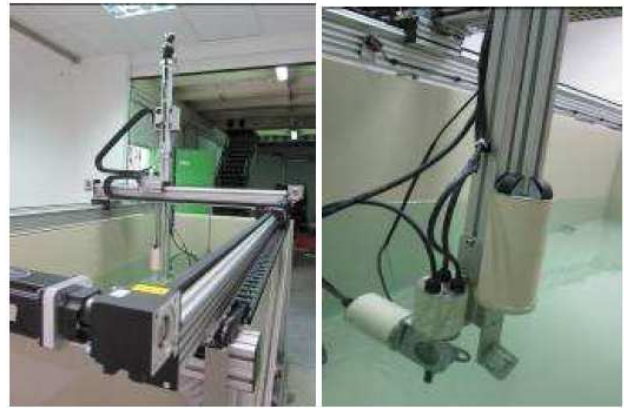
Fig. 25. VISIO water facility (2 m long, 1 m large, 1 m high) devoted to ultrasonic visualization study.
