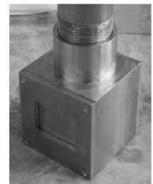
Fig. 2. Principle and photo of in sodium 8-phased array EMAT probe.
