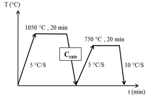
Figure 2: Applied heat treatment for microstructure generation
