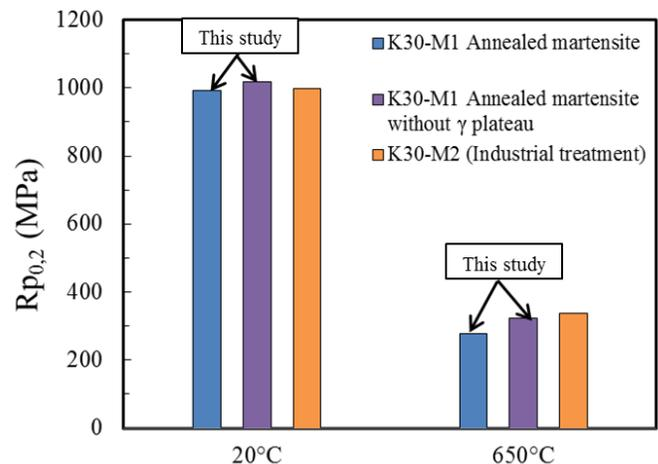
Figure 8: Yield strength comparison at 20°C and 650°C of different 9%Cr ODS steel cladding tubes investigated at CEA
