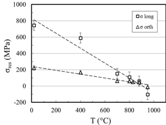
Figure 12: Macroscopic residual stresses evolution during the heat treatment
