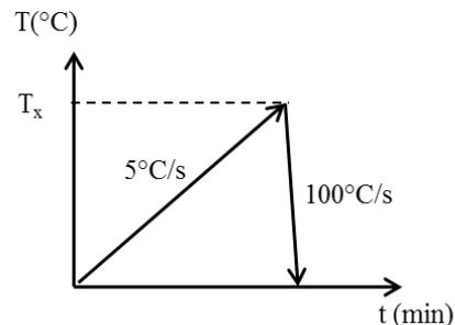
Figure 9: Applied heat treatment
