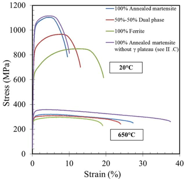
Figure 6: Tensile properties of the microstructures created using the dilatometer
