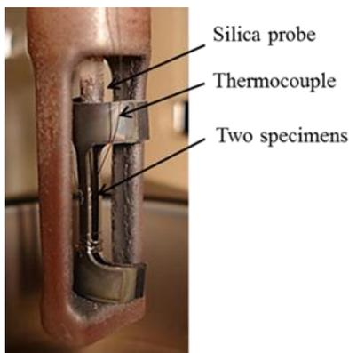
Figure 1: Experimental device
