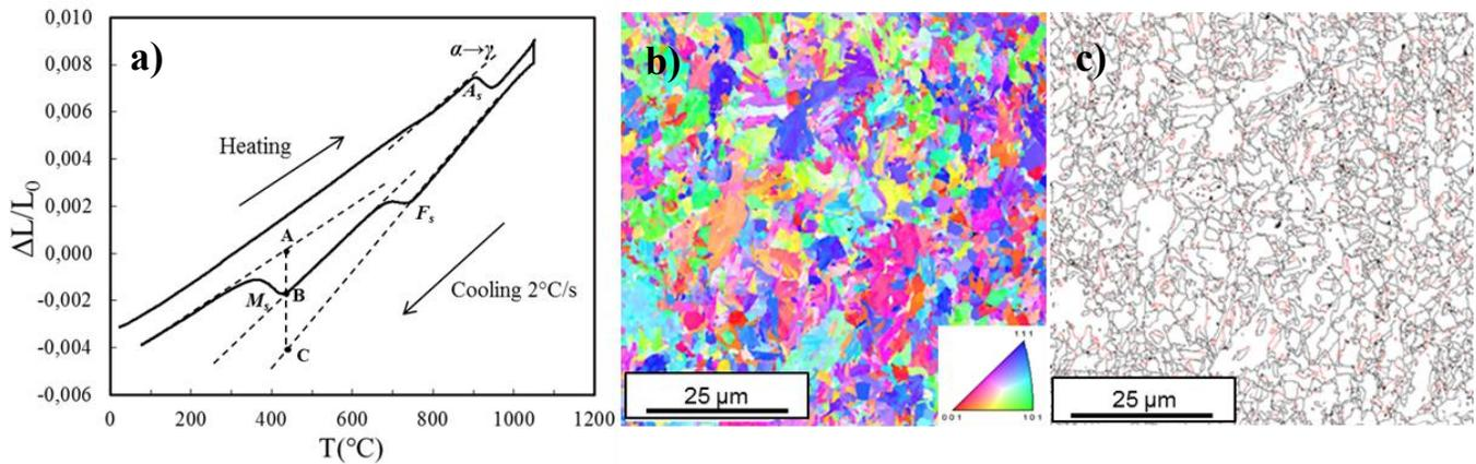
Figure 4: Dilation curve (a), Grain Orientation map (b) and Grain Boundaries Misorientation map (c) for the dual-phase microstructure
