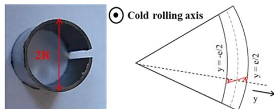
Figure 10: Orthoradial stress measurement
