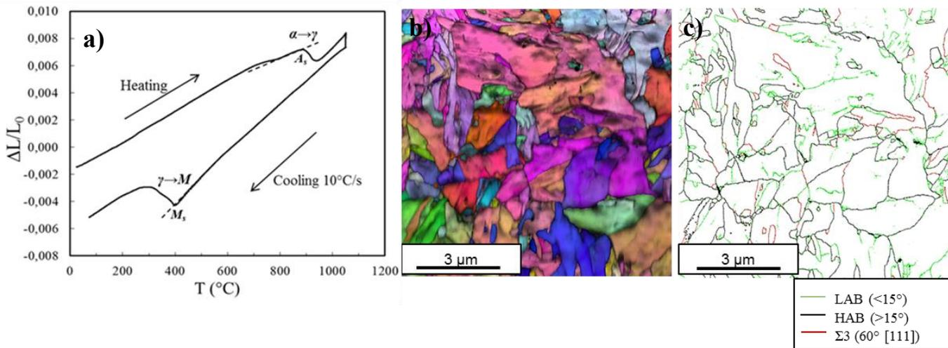
Figure 5: Dilation curve (a), Grain Orientation map (b) and Grain Boundaries Misorientation map (c) for the martensitic microstructure
