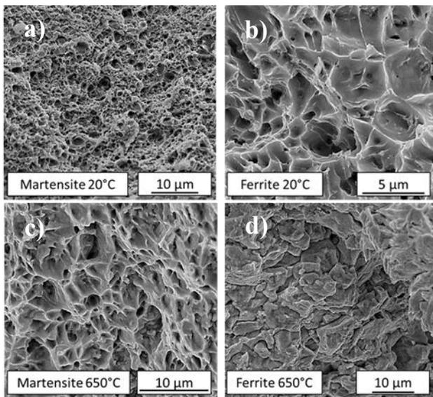
Figure 7: Fracture surfaces of tensile specimens
