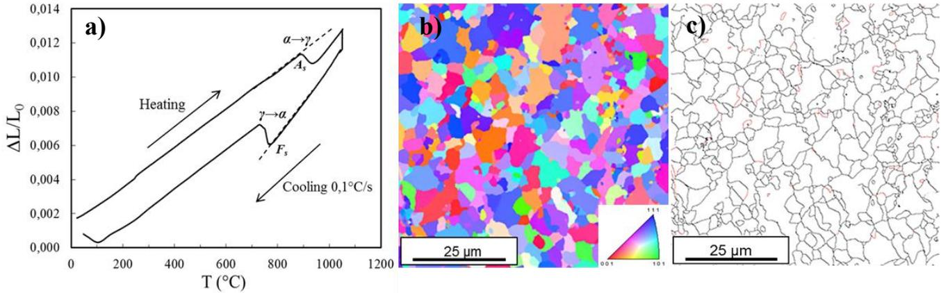
Figure 3: Dilation curve (a), Grain Orientation map (b) and Grain Boundaries Misorientation map (c) for the ferritic microstructure
