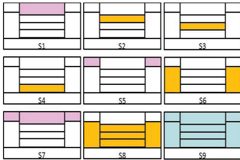
Fig. 4. Schematic representation of the core voiding scenarios: light violet indicates voiding of sodium plenum zones, amber—voiding of fuel zones and pale blue—total voiding, including inter-assembly gaps (IAG).
