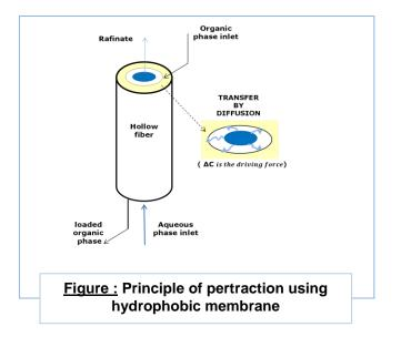
It is worth noticing that the aqueous-organic (aqueous-membrane) interface is essentially immobilized at the pore mouth of the hydrophobic membrane support through which the solute mass transfer takes place. It has several advantages over conventional solvent extraction method such as dispersion-free operation, very high contact surface area per unit extractor volume (provided by hollow fiber geometry), emulsion formation is avoided and nonrequirement of density difference of the phases.
