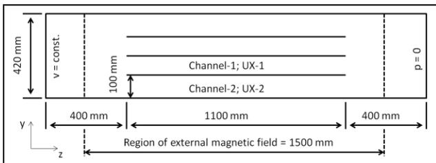
Fig. 5. Geometry of the EMIP model of TESLA-EMP.
