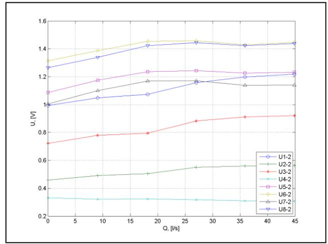
Fig. 25. 2<sup>nd</sup> coils signal,  $I = 200A$ :  $U = U(Q)$ .
