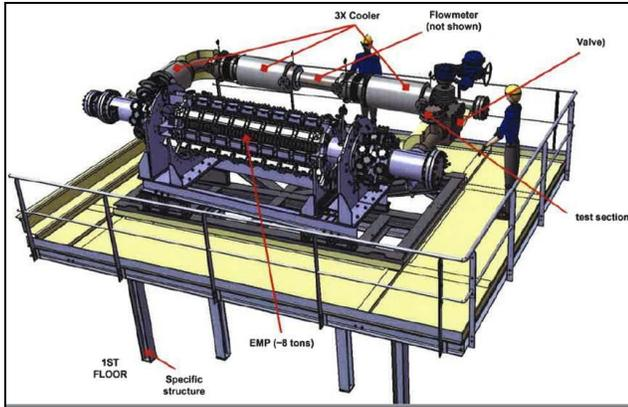
Fig. 1. A drawing of the PEMDYN facility.
