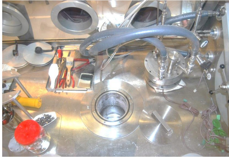
1- Liquid sodium, 2- Molybdenum crucible, 3- Thermal well, 4- Oven, 5- Cooling channels, 6- Gloves box floor, 7- Gas inlet and pressure monitoring, 8- Well cover, 9- Temperature well, 10- Upper cover cooling section, 11- Gas outlet, 12- Sodium vapor reflux condenser, 13- Aerosols filter, 14- Bursting disks, 15- Oxygen sensor, 16- Molybdenum wires, 17- Corrosion specimen
