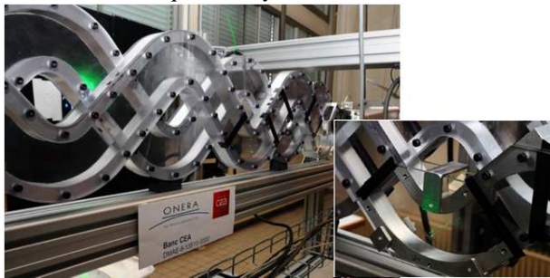
Figure 5: LDV device for aerodynamic validation
