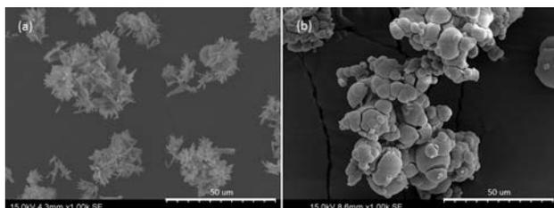
**Fig. 1.** SEM micrograph of neodymium (III) oxalate obtained (a) Without additive (b) In presence of NTMP
